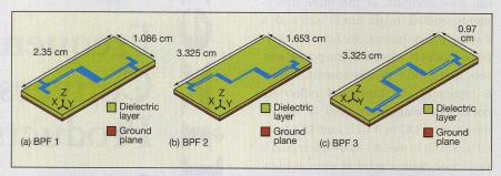
These three layouts show the topologies of the three UWB bandpass filters:
