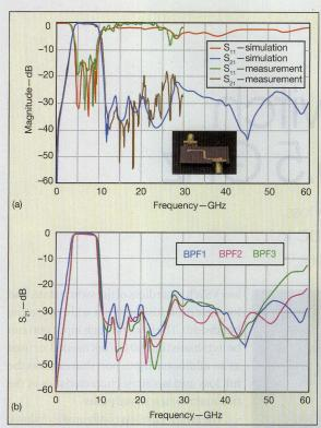
6. These plots show (a) the simulated and measured S-parameter responses as functions of frequency for the proposed UWB bandpass filter design, accompanied by a photograph of the fabricated filter as fabricated on commercial low-loss PCB material with relative dielectric constant of 2.20 and (b) a comparison of S-parameter responses for filters BPF 1, BPF 2, and BPF 3.
