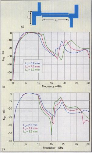
5. The schematic diagram of (a) the proposed coupling structure is shown next to (b) the simulated  $S_{21}$  responses for the proposed coupling structure with different values of  $L_2$  and (c) simulated  $S_{21}$  responses for the proposed coupling structure with different values of  $L_3$ .
