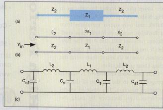
This schematic diagram of the stepped-impedance MMR
