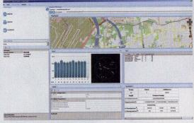
The HLTS test system works with the SimHybrid GUI to synchronize simulation or playback of A-GNSS, Wi-Fi, sensor, and cellular positioning technologies.
