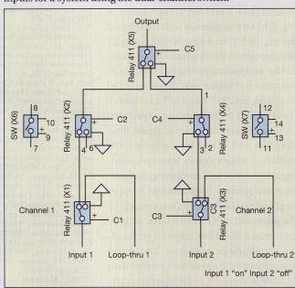
2. This schematic diagram shows the basic architecture of the loop-through switch.
