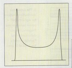
4. The model described by Harris and Warner has a U-shaped probability density function and is the model most widely used.
