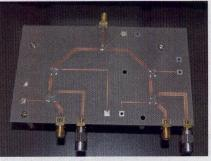
1. This is one possible circuit layout for the switch, fabricated on RT/duroid 5870 PCR material
