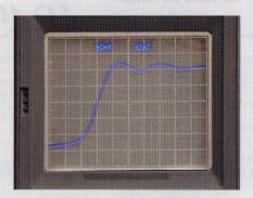
4. The two-channel switch circuit boasts excellent transient response, as shown by this oscilloscope display. The test signal source is a Tektronix S-52 pulse generator head with rise time of better than 25 ps, and the S-6 sampling head has a rise time of better than 30 ps.
