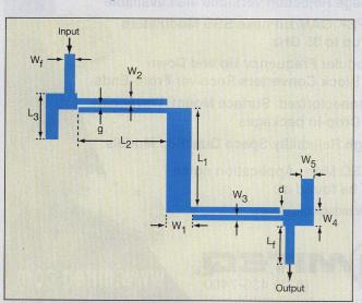
2. This layout shows the structural parameters for the proposed UWB BPF.
