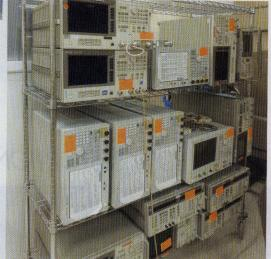
2. The effects from Sandy's floodwaters included damage to many of the RF/microwave vector network analyzers used for high-frequency production testing.
