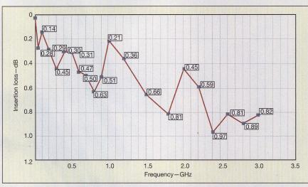
3. Insertion loss was evaluated through 3 GHz with level response across the full frequency range.
