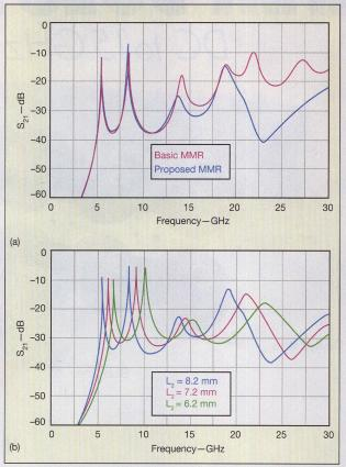
4. These plots show (a) the simulated  $S_{21}$  responses of the proposed and basic MMRs, and (b) the simulated  $S_{21}$  responses for the proposed MMRs with different values of  $L_2$ .
